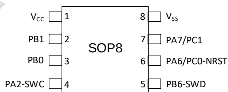
图 3-3 SOP8 Pinout1 PY32F002BL15S6-C (Top view)
